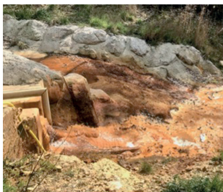
Figure 1 AMD stream and treatment device in-situ (polyethylene container).
