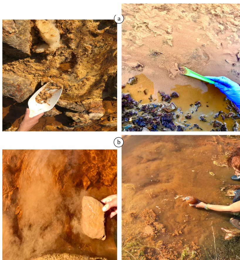
Figure 2 Sampling of precipitates in Acid Mine Drainage. a) Scrapping the substrate and b) slight agitation of the water for obtaining the flocculated material (fluffy precipitates).
