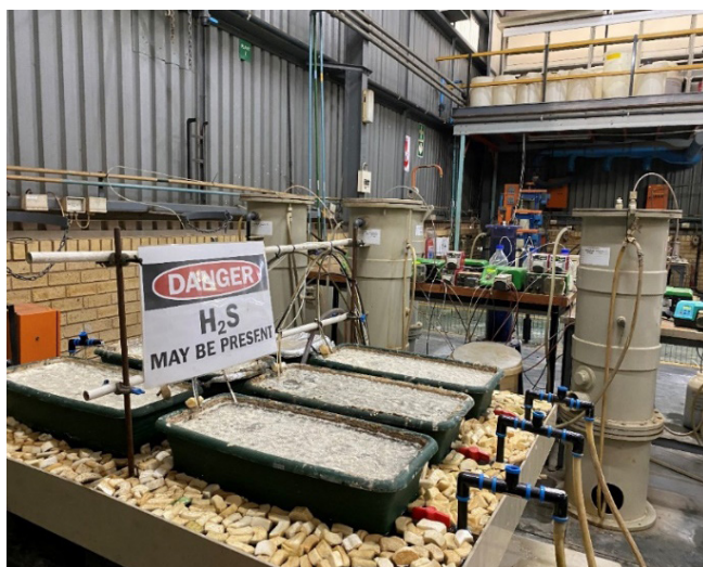
Figure 1 Photograph of Mintek's laboratory setup, the BSR columns are in the background and the sulfide oxidation tanks are in the foreground.
