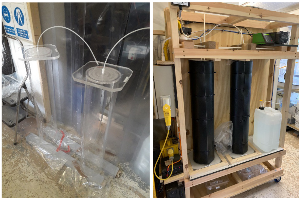
Figure 1 Laboratory columns and set-up (image: Geochemic Ltd).
