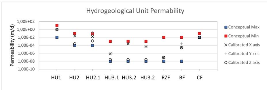
Figure 2 Conceptual and calibrated permeability for hydrogeological units
