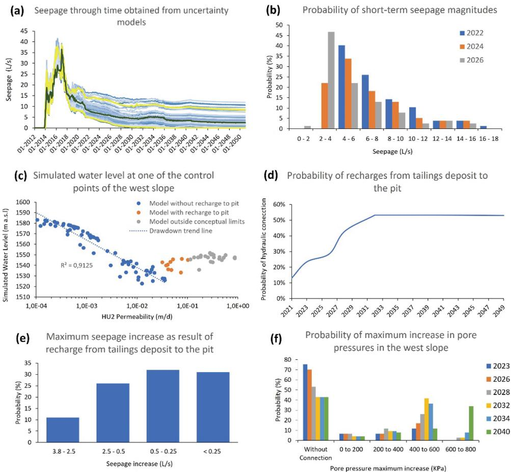
Figure 3 Results of uncertainty analysis. (a) Seepage over time; (b) Pit seepage magnitudes for short-term; (c) Correlation between drawdown in west slope water level and HU2 permeability; (d) Probability of recharges to reach the pit; (e) Magnitude of the maximum seepage increase; (f) Increase of pore pressure through time
