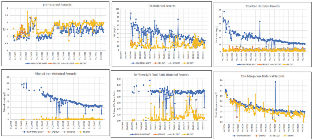
Figure 1 Monitoring data from shaft mine water (raw from shaft), outflow from settlement ponds (SP1/2 OUT) and final discharge post reed beds (RB OUT). Monitoring data for the period 2004 to 2021. Source: The Coal Authority
