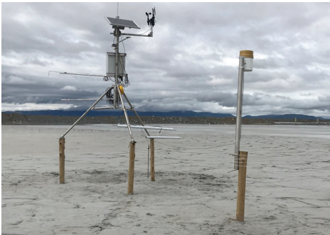
Figure 3 Surface Renewal station at the start of the observations
