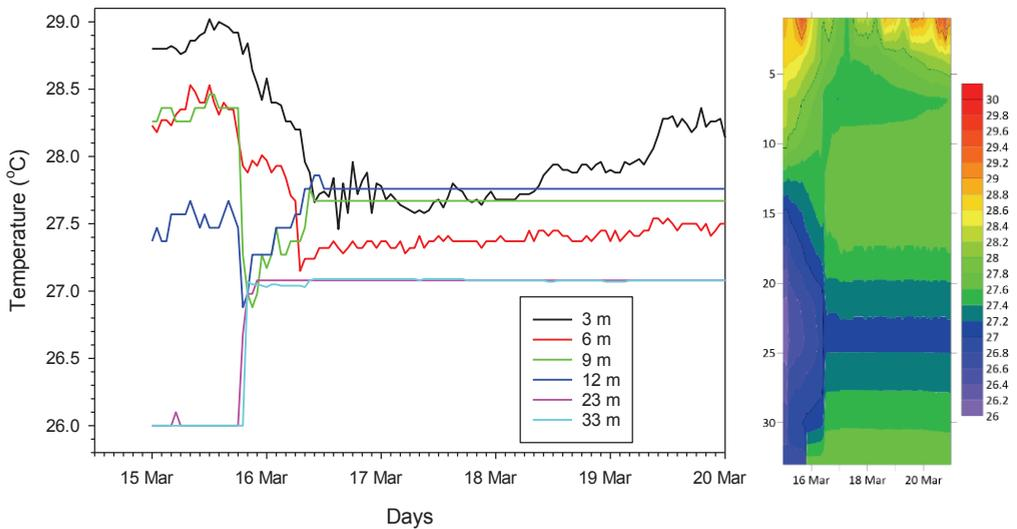
Figure 4 Water temperatures with depth at BL1 before and after the 100 mm rain event (on 15 March 2019).
