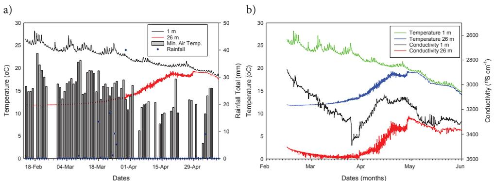
**Figure 2** In 2019 for HL1, a) water temperatures at surface (1 m) and bottom (26 m), with minimum daily air temperatures (Gulgong Post Office, BOM 2020) and daily rainfall (Ulan Water, BOM 2020) between February and May and b) water temperature (1 and 26 m) and conductivity (surface and bottom; inverted axis – to reflect increasing water density) for the winter mixing event
