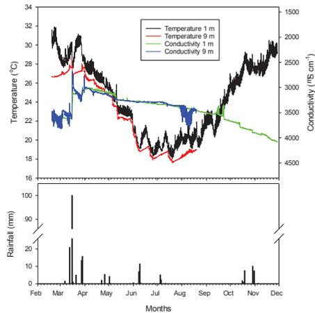
Figure 3 Daily rainfall, and surface (1 m) and bottom (33 m, 9 m respectively) conductivity and temperature in a) BL1 and b) BL2 in 2019 (Note the inverse conductivity scale to reflect density).
