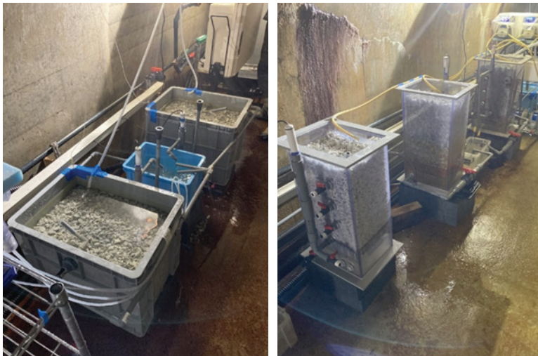
Figure 2 Reactors employed in the continuous flow test; limestone reactor (right), CWM reactor (left)
