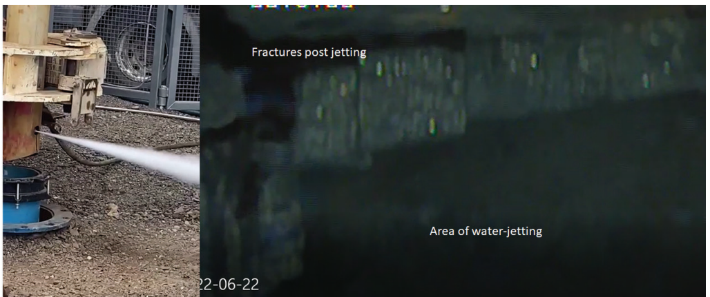
Figure 3 Water jet test at surface (left), and borehole CCTV image post-water jetting (right). Photograph from Integrated Water Services and European Geophysical Services
