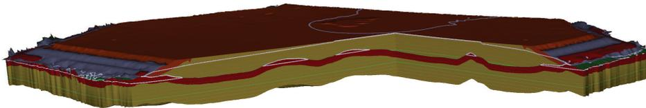
Figure 1 Section of a Ghanaian TSF integrated into a numerical groundwater model
