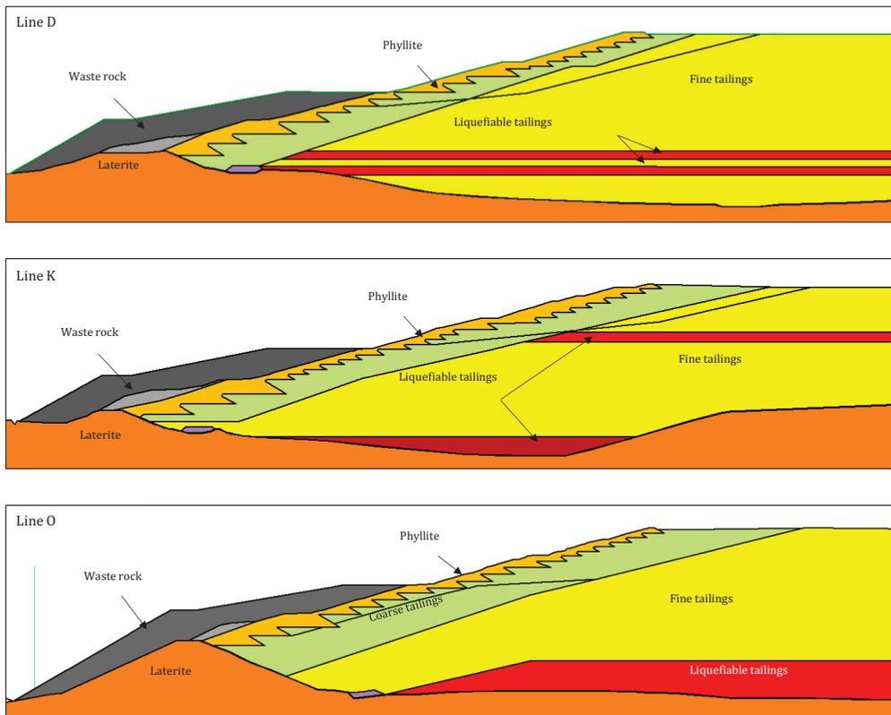
Figure 4 Zones of liquefiable tailings identified in a Ghanaian tailings storage facility
