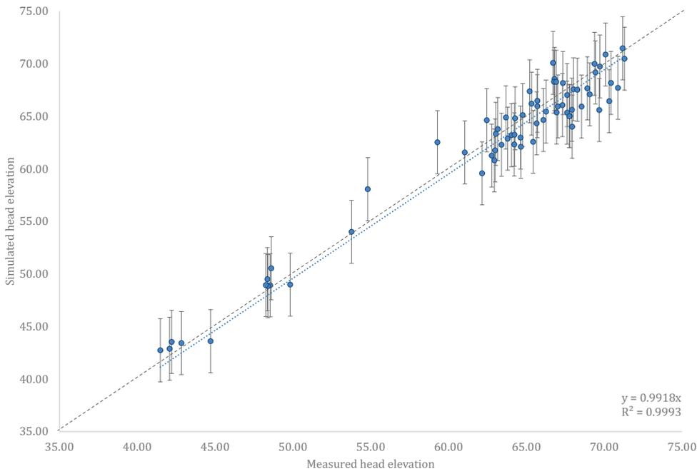
Figure 2 Calibration graph of measured hydraulic head elevations compared to simulated hydraulic head elevations for a South African gold tailings storage facility
