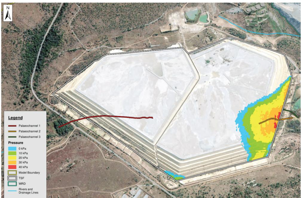
*Figure 3 Elevated hydraulic pressure zones due to groundwater influx at the base of a South African gold tailings storage facility*
