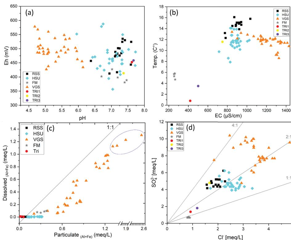
**Figure 1** a) Eh-pH diagram; b) Temperature versus electrical conductivity diagram of the Erzgebirge mine waters; c) Ratio of Particulate to dissolve Al+Fe; d) The relationship between Chloride and Sulfate (Rothschönberger Stollen – RSS; Hauptstolln Umbruch – HSU; Königliche Verträgliche Gesellschaft Stollen – VGS; Freiburger Mulde – FM; Triebisch River –Tri).
