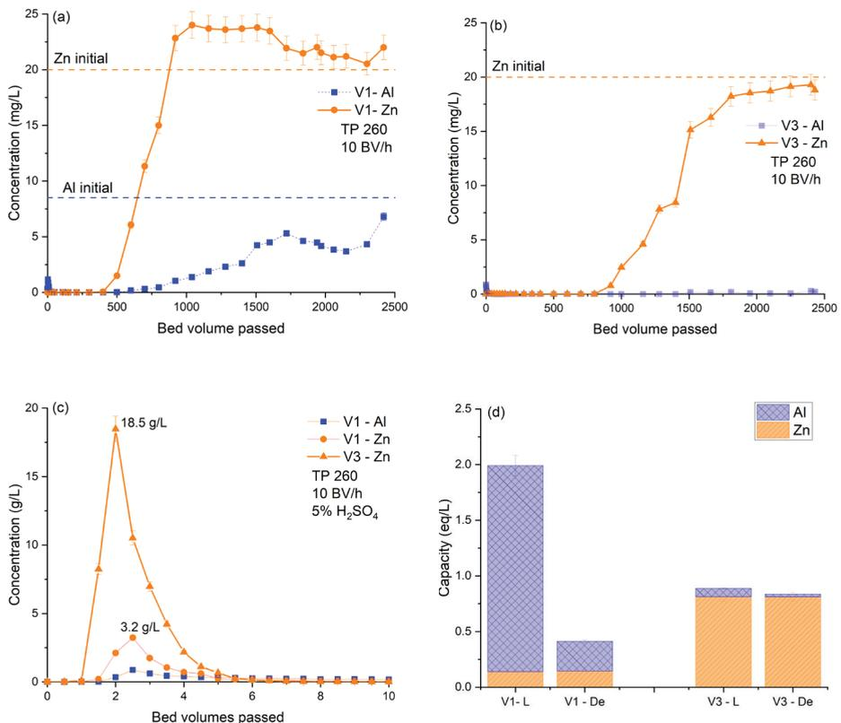
**Figure 1** a) Breakthrough curves of untreated mine water (Zn and Al) loaded into IX column with TP 260 resin; b) breakthrough curves of pretreated mine water (after Al precipitation); c) De-loading curves of Zn and Al in untreated (column A) and pretreated (column B) mine waters; d) Mass balance of column A and B (L-loading, De-De-loading).
