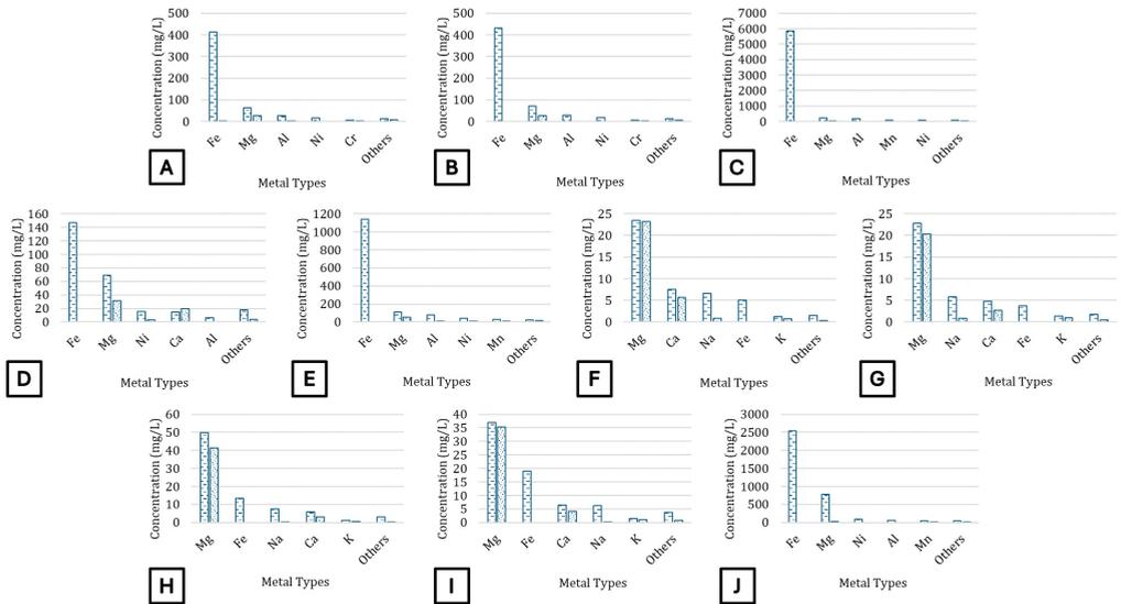
Figure 5 Characteristics of Total Metals in the Wet Season: Pond 1 (A), Pond 2 (B), SS9 (C), SP1 (D), SP4 (E), MEM A (F), MEM B (G), Mine A (H), Mine B (I), and Slag (J).
