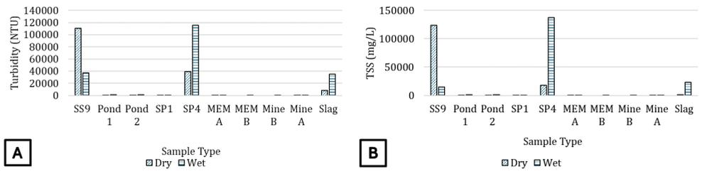
Figure 3 Comparison of turbidity (A) and TSS (B) in each sample.
