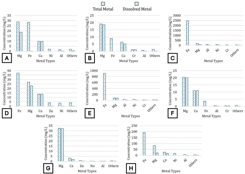
Figure 4 Characteristics of Total Metals in the Dry Season: Pond 1 (A), Pond 2 (B), SS9 (C), SP1 (D), SP4 (E), MEM A (F), Mine A (G), and Slag (H).
