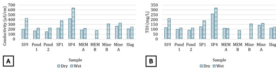
Figure 2 Comparison of conductivity (A) and TDS (B) in each sample.
