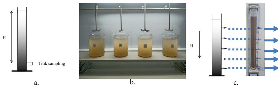
Figure 1 Illustration of (a) type 1 of sedimentation test, (b) jar test, and (c) type 2 of sedimentation test.
