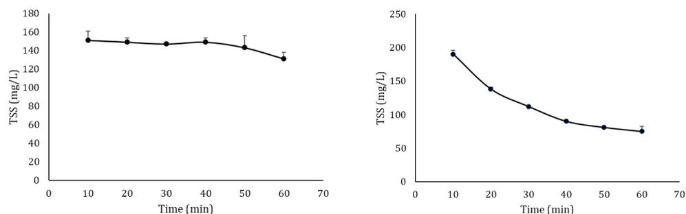
Figure 2 Variation in TSS concentration over settling time in type 1 of sedimentation (discrete particle) for: a. sample with high turbidity (A03) and b. sample with acidic pH and high turbidity (B07).
