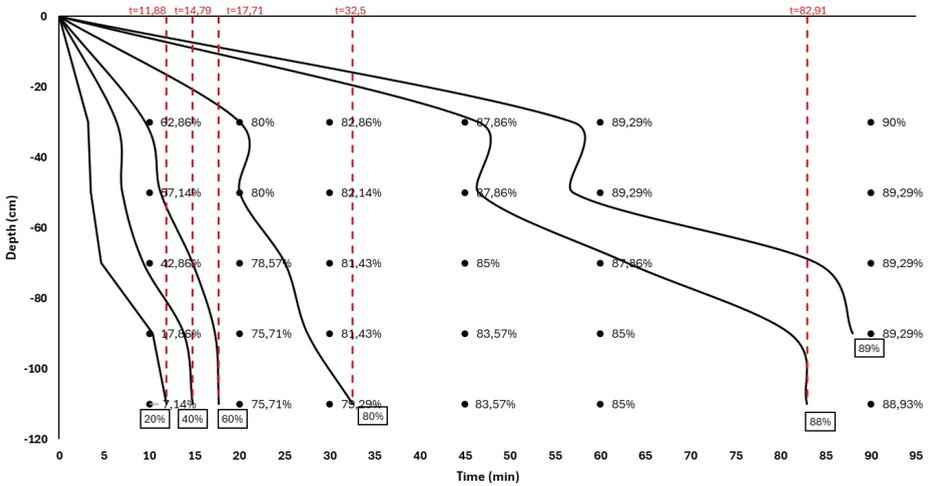
Figure 3 Iso-removal graph for sample A03 with a target efficiency of 82.14% (achieving the water quality standard of 100 mg/L TSS concentration).
