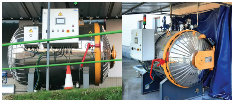
Figure 1 Reactor for hydrochar production utilising the residual steam flow from the electricity generation of the hospital waste incinerator at COGERSA (image: Álvaro Amado-Fierro).
