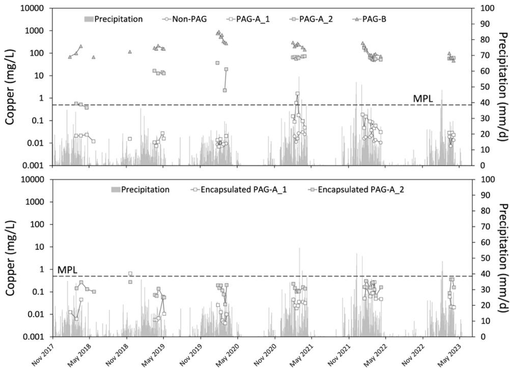
Figure 3 Graphics showing the geochemical evolution of some of the field humidity cells. Upper graphic shows the evolution of cells representative of the three GEUs, whereas bottom graphic shows the evolution of two of the cells where a 0.5 m thick layer of PAG-A material was sandwiched between two 0.25 m thick layers of Non-PAG material. Histogram at the bottom of both graphs represents the daily precipitation MPL: maximum permissible limit.
