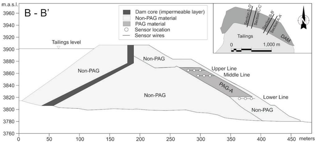
Figure 2 Profile across the dam of the tailings facility showing the PAG layer and the location of the sensors.
