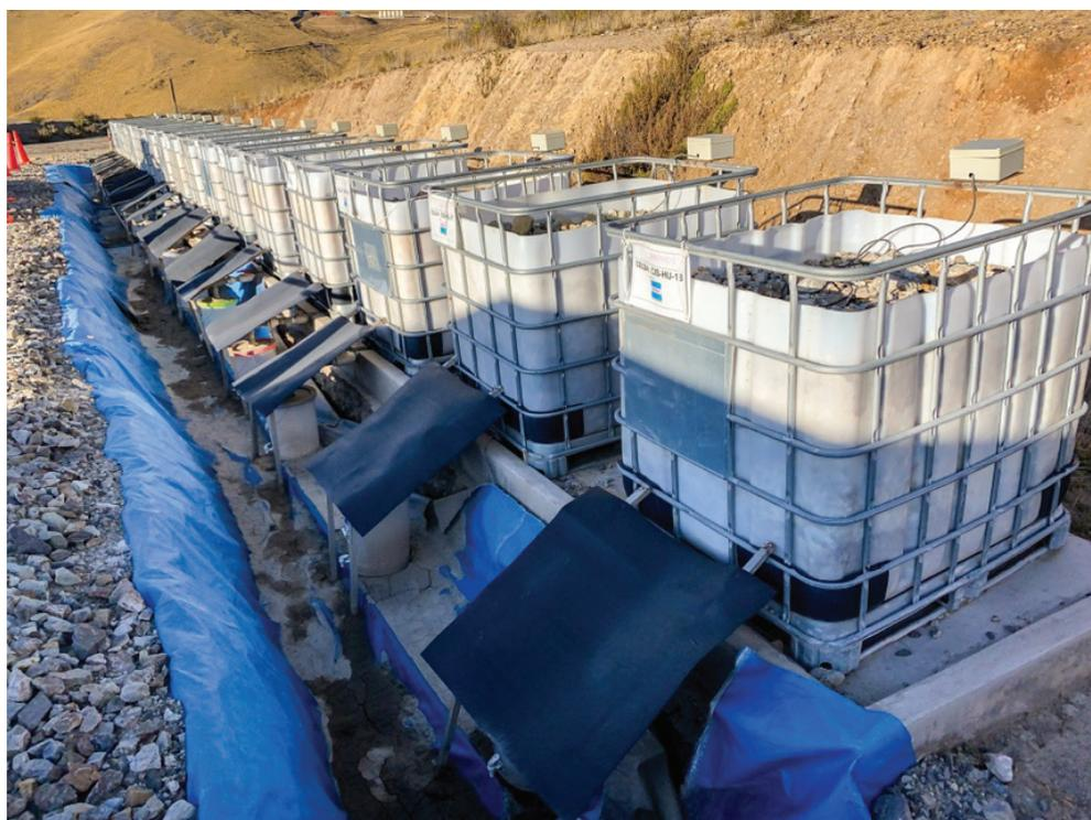
Figure 1 Field humidity cell tests at the mine site.
