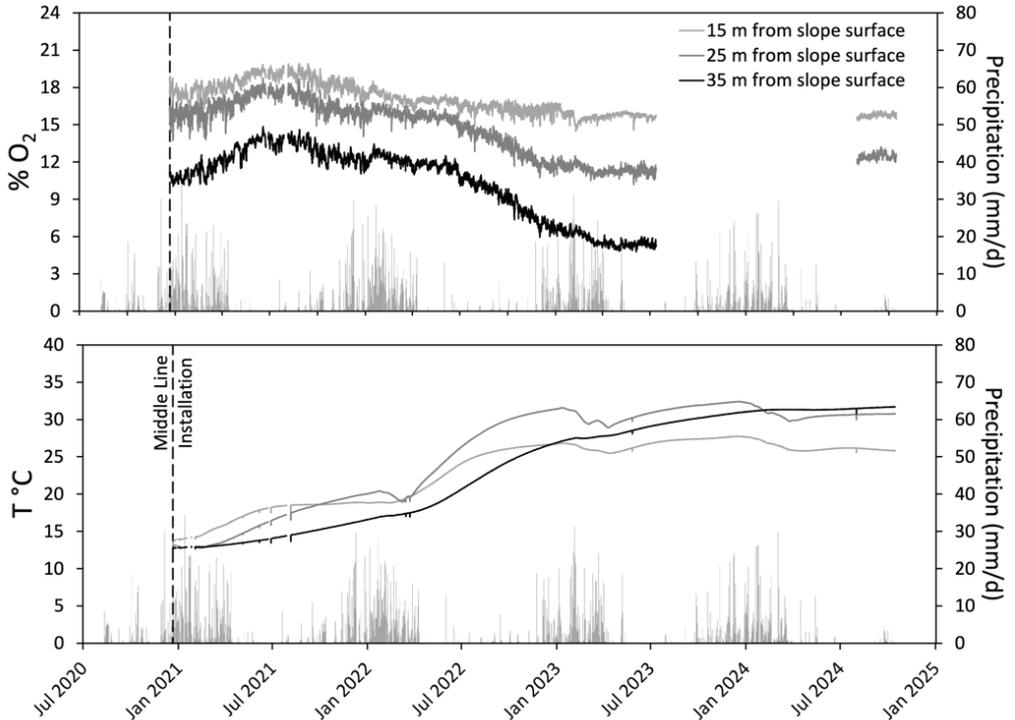
Figure 4 Graphics showing the evolution of oxygen in the gas phase and temperature measured by sensors in one of the middle lines installed in the tailings dam.
