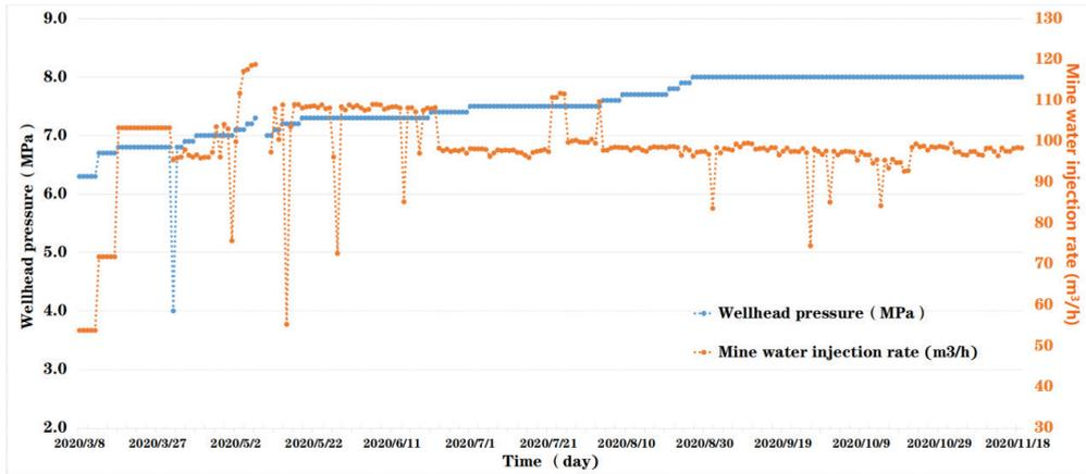
Figure 3 Wellhead pressure and injection flow rate for MC-1 well.
