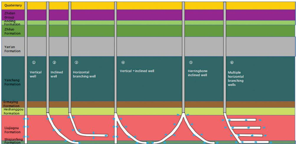
Figure 2 Different well constructions for mine water injection and storage.
