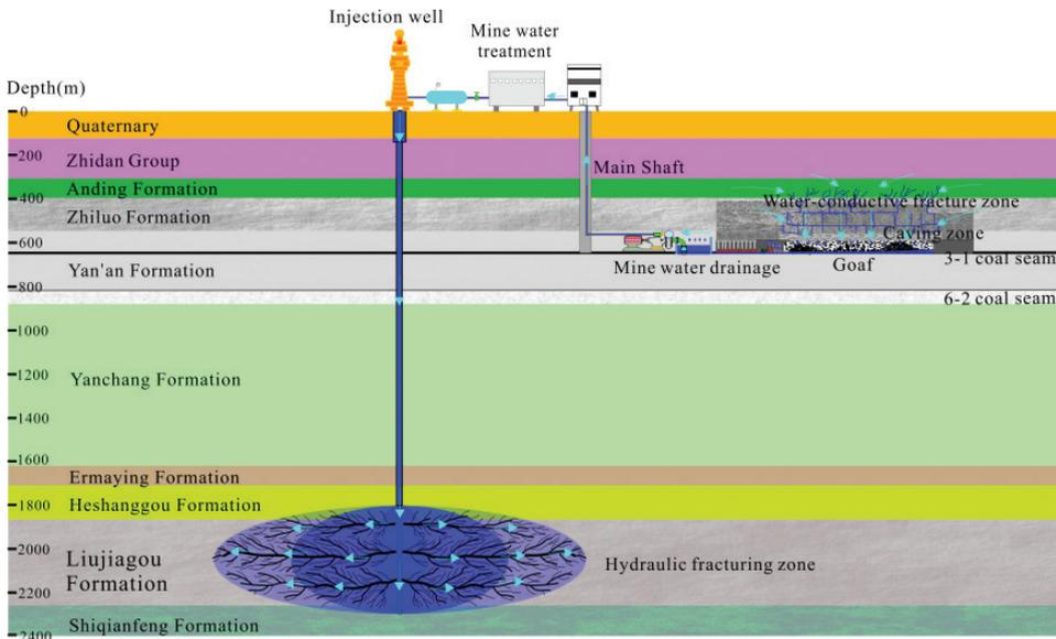
*Figure 1 Schematic diagram of the typical hydro-geological framework of mine water injection and storage in the deep sandstone aquifer.*
