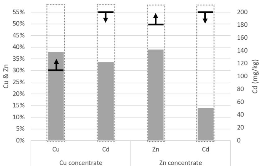
**Figure 2** Cu, Zn, and Cd concentrations in concentrate compared to target values. The arrows indicate threshold requirements: Cu and Zn concentrations must meet or exceed the target, while Cd concentrations must remain below the target.
