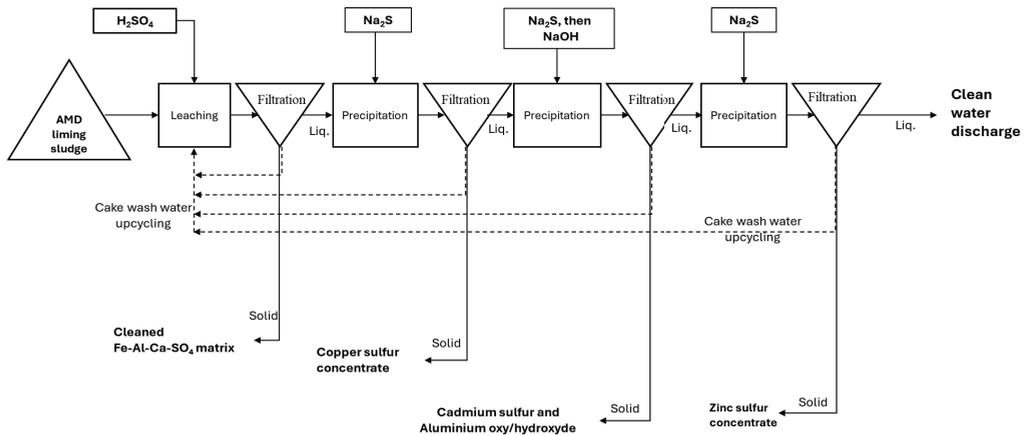
Figure 3 Process flowsheet for selective leaching and precipitation of Cu, Zn, and Cd from AMD liming sludge.
