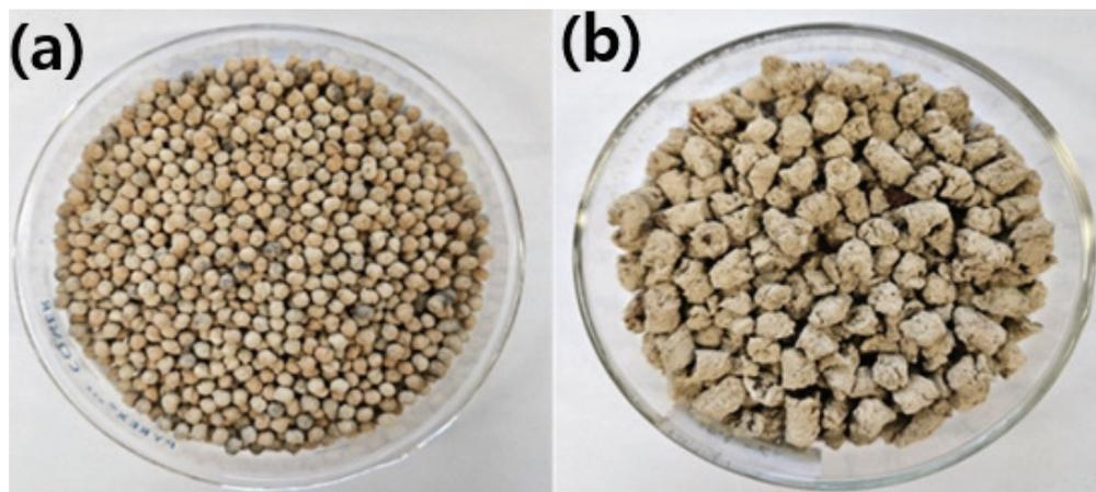
*Figure 1 Photographs of the adsorbents used in the secondary treatment process: (a) adsorbent made from sludge of a domestic water purification facility and (b) from sludge of a coal mine drainage treatment facility.*
