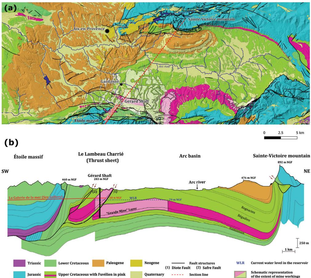
Figure 1 Simplified geological map (a) and cross-section (b) of the Gardanne basin, illustrating the main lithological units and structural features; (b) adapted from J-P Durand (1980, *Houillères du Bassin de Centre-Midi*) (NGF: French altimetric reference based on the mean Mediterranean Sea level).
