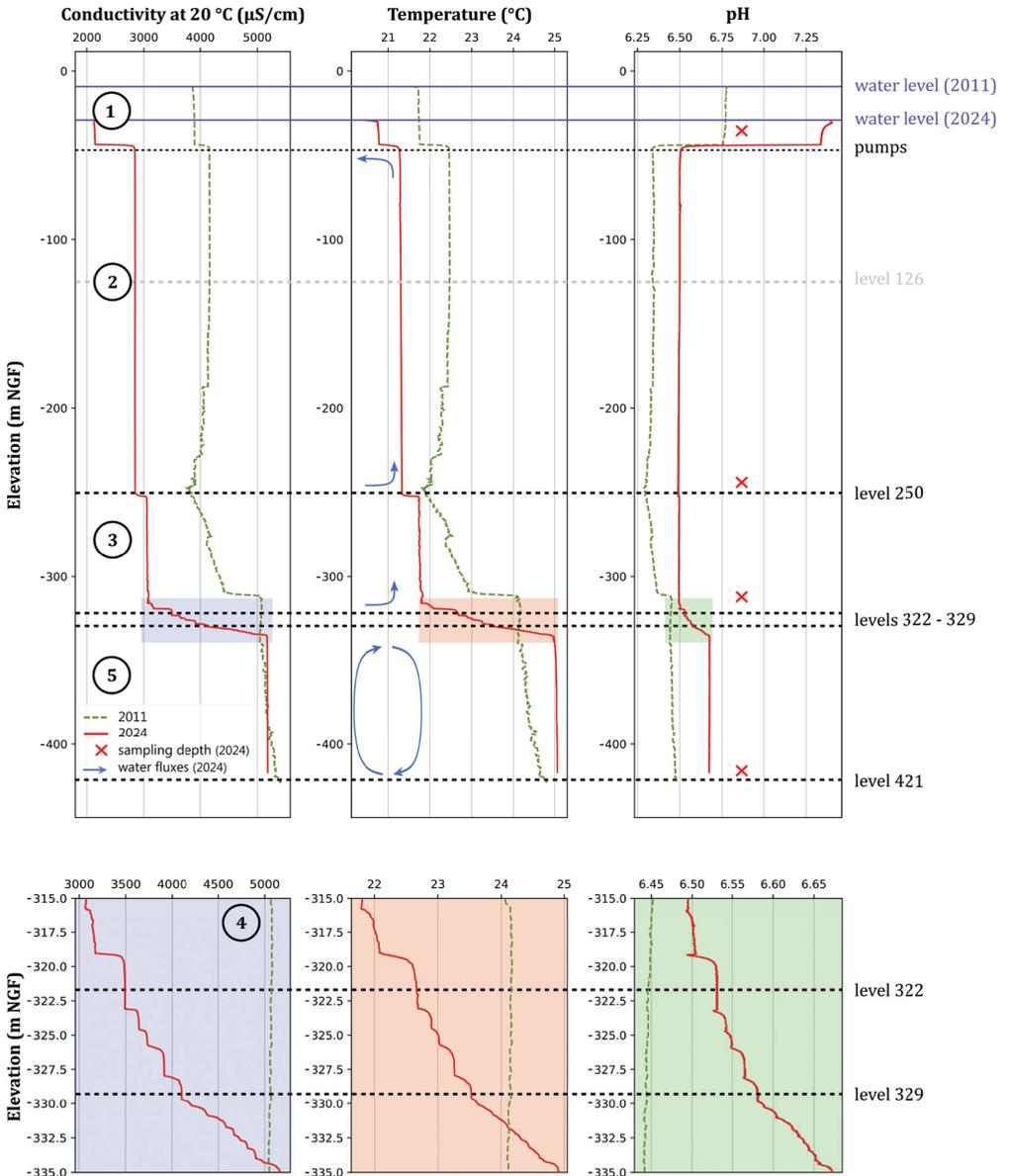
Figure 2 Comparison of pH, Conductivity and Temperature logs in the Gérard Shaft (2011 & 2024).
