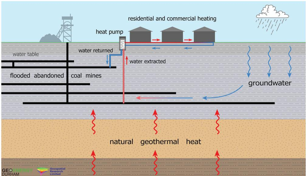
**Figure 1** Schematic overview on how to utilise mine water for geothermal heating (from Geospatial Research Ltd. 2025).
