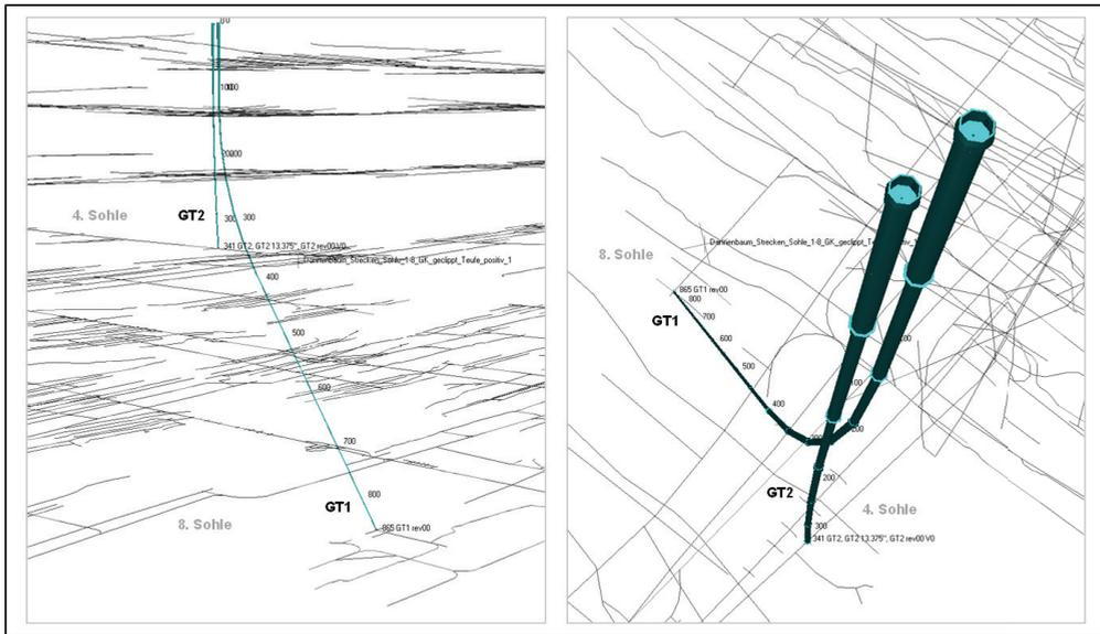
Figure 2 Directional wells GT1 & GT2 at Dannenbaum colliery (Hahn 2024a).
