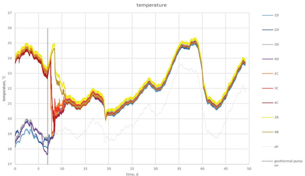
**Figure 4** Temperature curve before and after the geothermal pump was switched on (dotted line) with probes above level 145 (1D, 2D, 3D, 4D) and probes below level 145 (2C, 3C, 4C, 2B, 4B).
