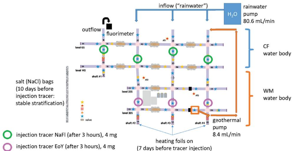
Figure 3 AMM set-up of the experiment with tracers Sodium Fluorescein (NaFl) and EosinY (EoY).
