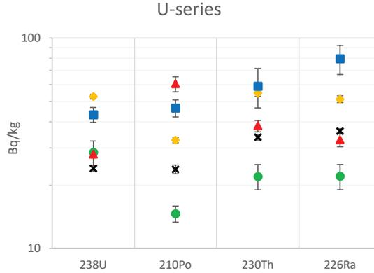
Figure 3 <sup>238</sup>U series activity concentrations of pyrite flotation (FP), pyrite roasting (RP), smelting slags (SL), leached pyrite (PY) and shale rejects (SH).
