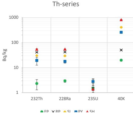
Figure 4 <sup>232</sup>Th series and <sup>40</sup>K activity concentrations of pyrite flotation (FP), pyrite roasting (RP), smelting slags (SL), leached pyrite (PY) and shale rejects (SH).
