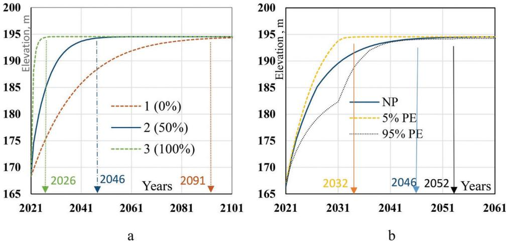
Figure 4 Prediction of Kopeysk open pit flooding for different scenarios allowing for: a degree of pit backfilling (1—without backfilling, 2—with 50% backfilling, 3—with 100% backfilling); b variation in natural water recharge (1—normal period (NP), 2—water-rich period with 5% probability of excess for 10 years (5% PE), 3—water-short period with 95% probability of excess for 10 years (95% PE). The number at the arrow means the year of peak water mark.
