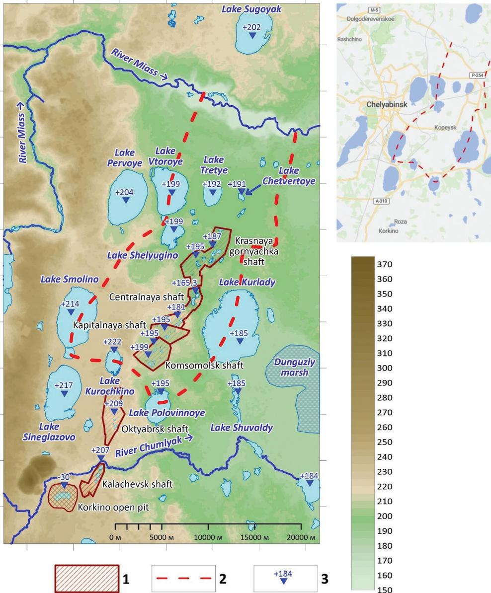
Figure 2 Hydrographic network of the region and minefield location map. 1 – mining allotment; 2 – mine catchment area boundary in the northern part of the Chelyabinsk Coal Basin (groundwater flow model boundary); 3 – reservoir water level mark.
