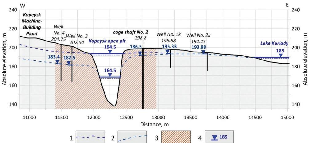
**Figure 3** Schematic cross section along the line Kopeysk Machine-Building Plant – Kopeysk open pit – Lake Kuraldy. 1 – current groundwater level; 2 – predicted groundwater level; 3 – mining allotment for the shaft Tsentralnaya; 4 – absolute water-level elevation.
