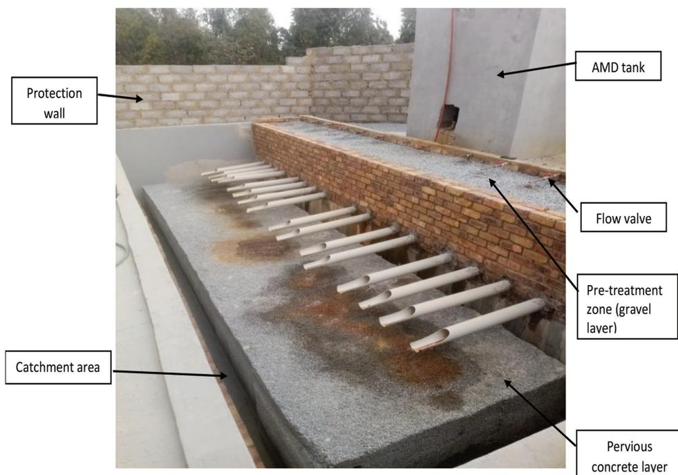
Figure 1 Pervious concrete reactive barrier system.
