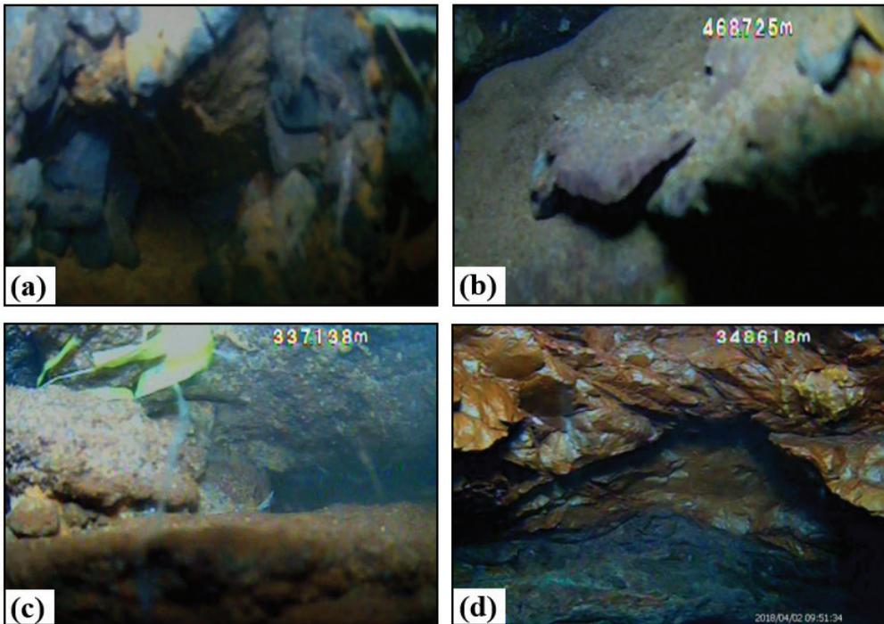
Figure 3 Borehole TV and ultrasonic imaging reveal bed separation and fracture development.
