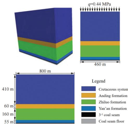
**Figure 1** Numerical simulation model of the panel 11-3101.
