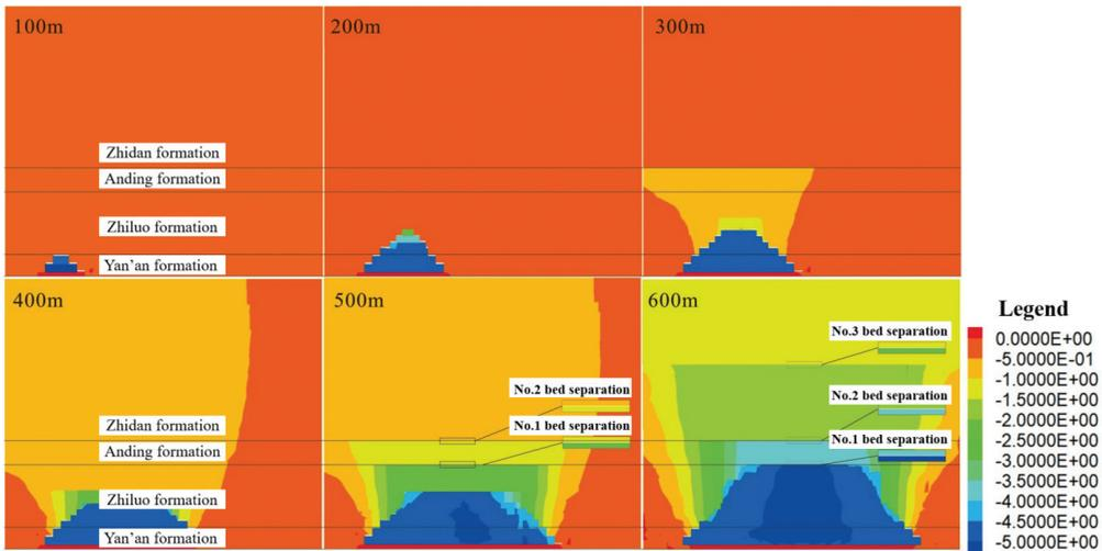
Figure 2 Vertical displacement of overburden rock of the panel.
