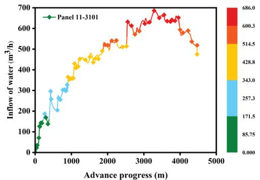
Figure 5 Water inflow curve in the panel.
