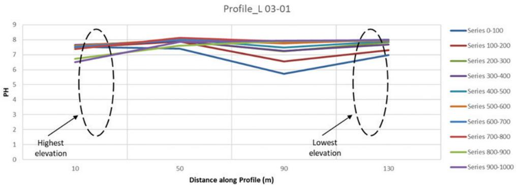
Figure 5 Example cross section of paste pH in thickened tailings underneath waste rock cover. Values in the legend refer to 100-mm depth increments of each sample below ground surface.
