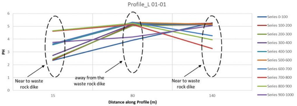
Figure 4 Example cross section of paste pH in uncovered thickened tailings. Values in the legend refer to 100-mm depth increments of each sample below ground surface.
