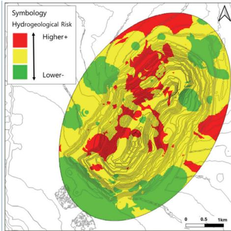
Figure 4 Hydrogeological risk map associated with slope stability in the open pit.
