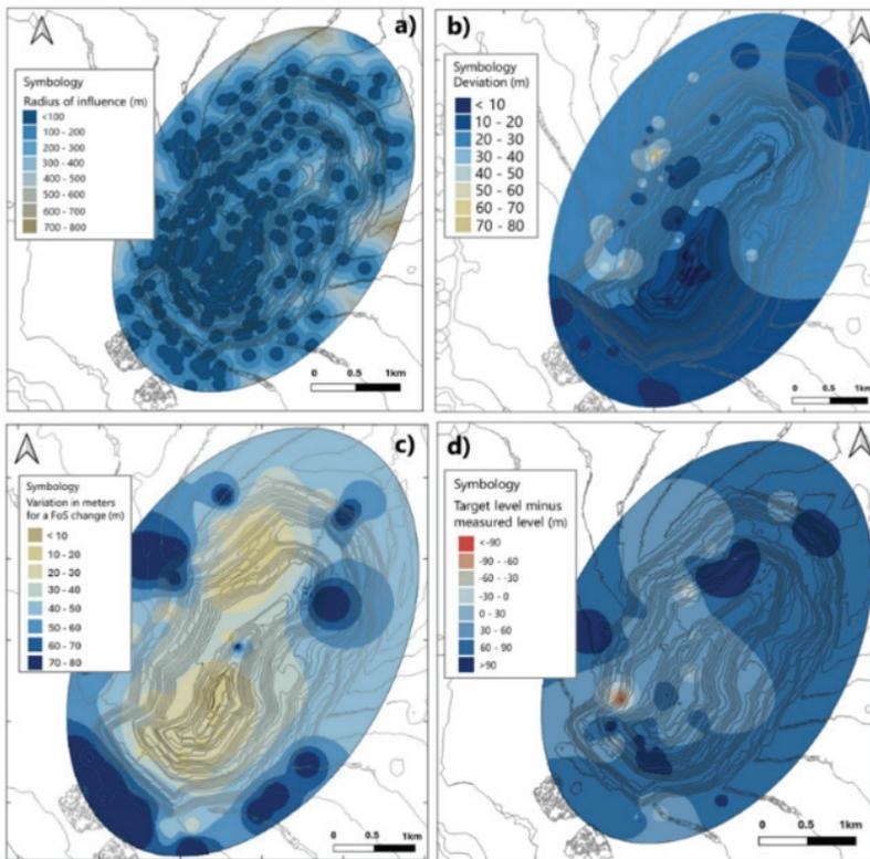
**Figure 1** Maps used to generate the Hydrogeological Risk Map associated with slope stability in the open pit. a) Information density map, b) Deviation level for 80% of the uncertainty models (P80), c) Slope stability sensitivity to the pore pressure and d) Difference between target level and measured level.
