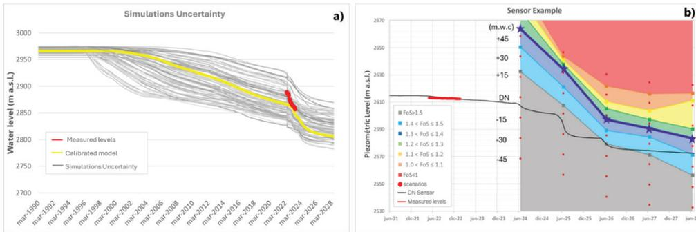
Figure 2 Uncertainty analysis and impact of pore pressure on slope stability: a) Uncertainty simulations, measured level, and best-calibrated model. b) TARP chart linking the water table level to the Factor of Safety.
