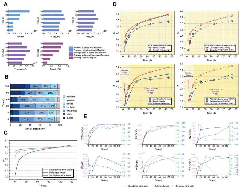
**Figure 3** Soaking test results, (a) data of pore fracture parameters of coal sample under different soaking duration; (b) mineral composition ratios of coal samples at different soaking time; (c) pH value of soaking solution changed with different soaking time; (d) mechanical damage coefficient under different soaking conditions; (e) The ion concentrations in different soaking solutions change with different time, respectively.
