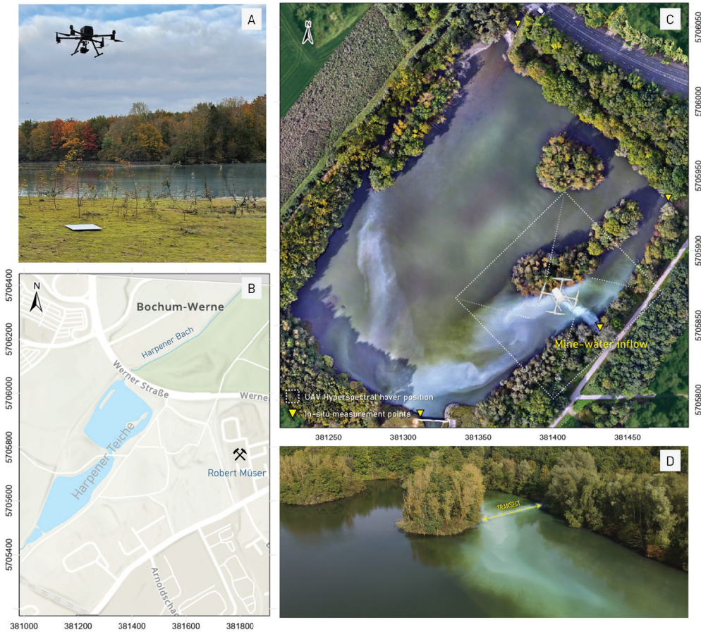
Figure 1 Study area and UAV monitoring configuration at Harpener Teiche (Bochum, Germany). (A) UAV system used for hyperspectral data acquisition. (B) Location within Bochum. (C) UAV orthomosaic showing the mine-water inflow, hover acquisition area, and in-situ measurement points (yellow markers). (D) Oblique image of the visible plume and the A–B transect used for spatial analysis. Coordinates in panels B and C: ETRS89 / UTM Zone 32N (EPSG:25832), in meters.
