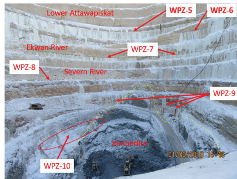
Figure 2 a) cross section illustrating general stratigraphy at the open pit (above), and b) 2019 picture from open pit showing inflow from individual water producing zones in lower portion of open pit (right).
