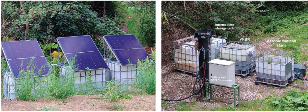
Figure 5 Pilot plant setup: PV modules and storage IBC (left), process stages: travertine filter, intermediate storage, vertical flow bioreactor (VFBR) and plant basin (right).
