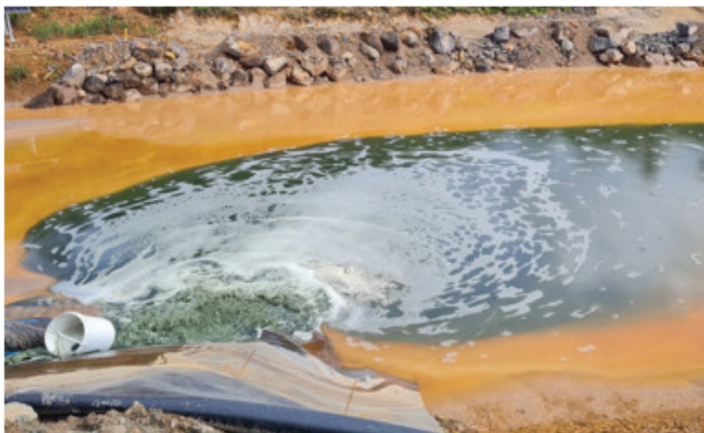
Figure 1 Green-blue colouration within treated “Sample 1” AMD, dosed with hydrated lime to pH 4.5.
