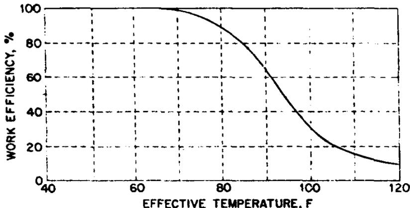
FIG. 7. EFFECTIVE TEMPERATURE AND WORK EFFICIENCY.
