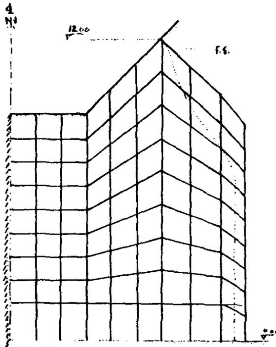
Fig. 11 (3rd. Ex.) - Flow out of a ditch.
