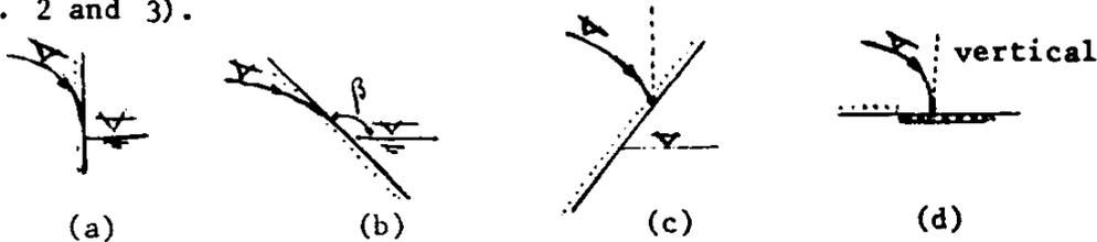
Fig. 2. Intersection of a phreatic surface with seepage face (isotropic media)
