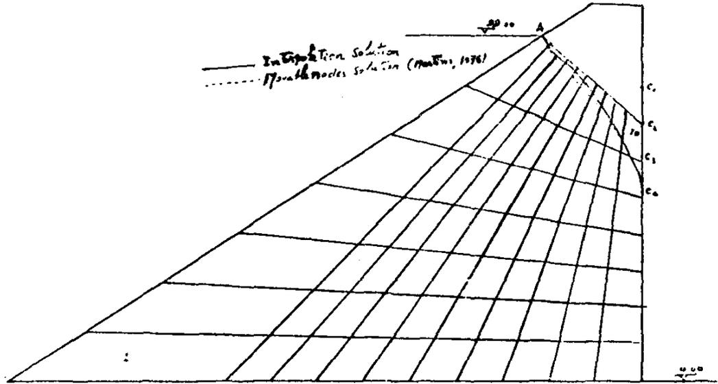
Fig. 9 (1st. Ex.) - Homogeneous dam with vertical filter. F.E. mesh.
