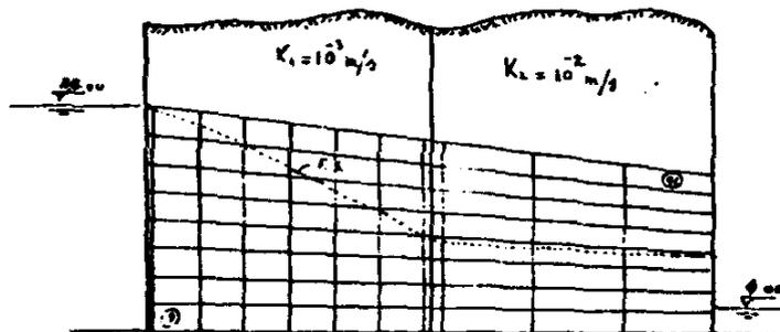
Fig. 12 (4th. Ex.) - Seepage through heterogeneous aquifer. F.E. mesh.
