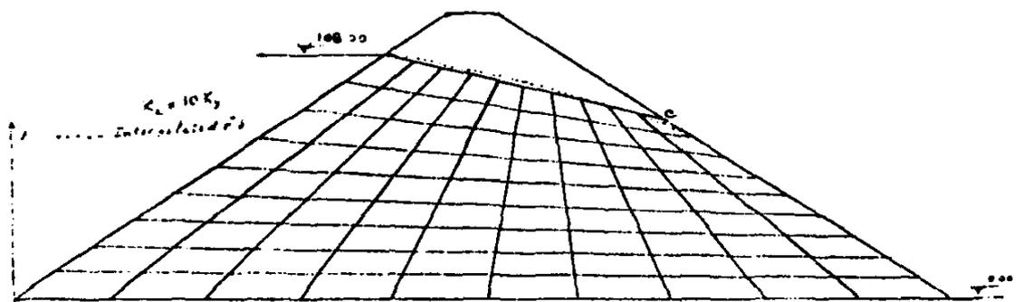
Fig. 10 (2nd. Ex.) - Anisotropic dam F.E. mesh. No flow on F.S. after determination of exit point C.
