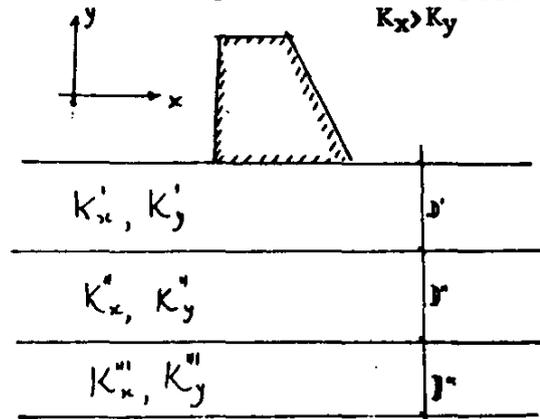
Fig.6 - Anisotropic heterogeneous layered medium
