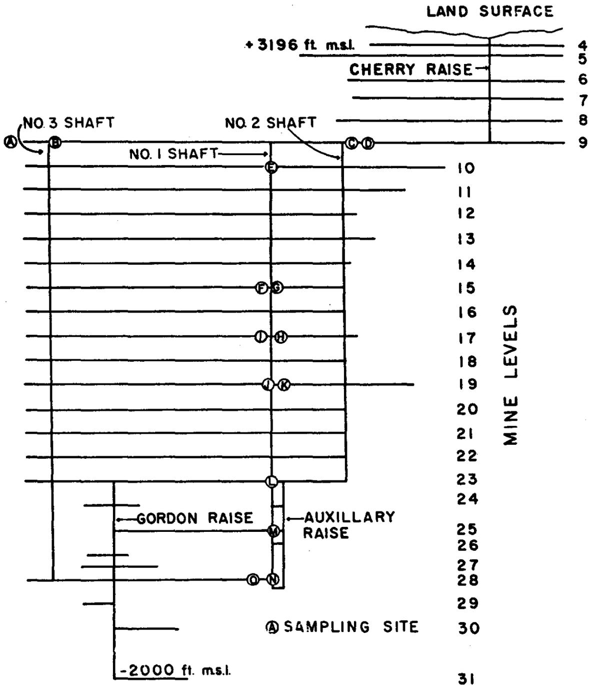
Figure 4. Generalized diagram of the Bunker Hill Mine showing location of sampling stations in the Mine's pumping system.
