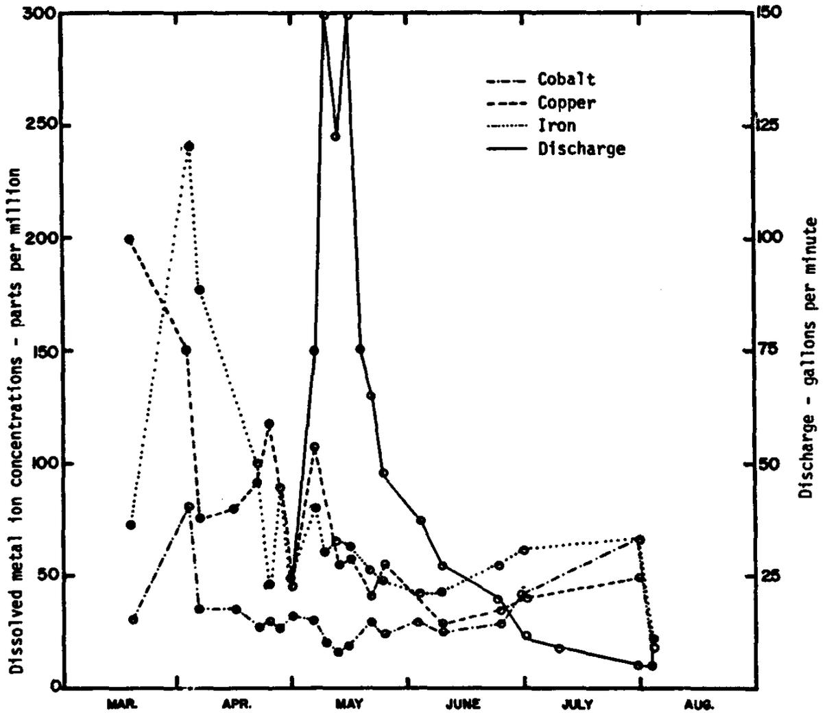
Figure 2. Dissolved cobalt, copper, and iron concentrations at station 10 (7100 waste pile) for 1976.
