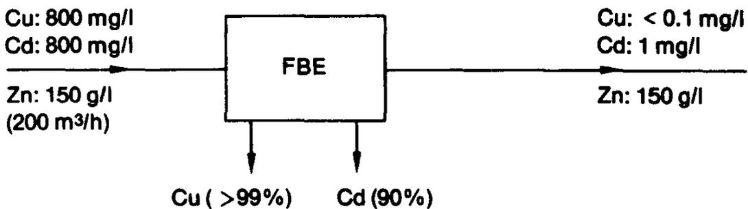
**Figure 12. Copper-cadmium Removal from Zinc Electrolyte by Means of Zinc Dust Cementation (A) and Fluidized Bed Electrolysis (B)**
