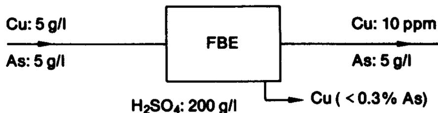
Figure 11. Copper-Arsenic Separation without AsH<sub>3</sub> Evolution
