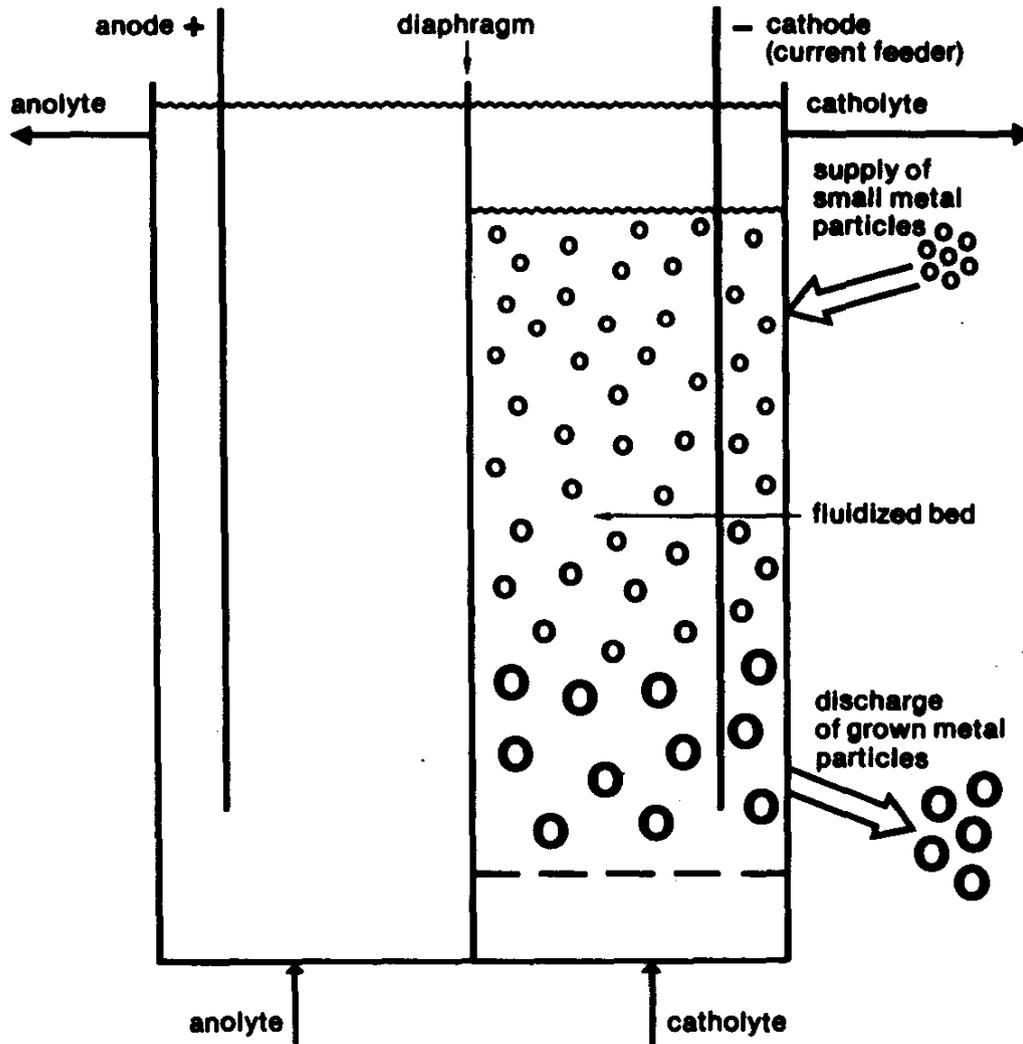
Figure 2. Schematic View of an FBE Cell
