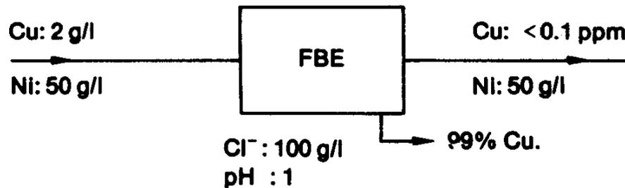
Figure 10. Copper-Nickel Separation
