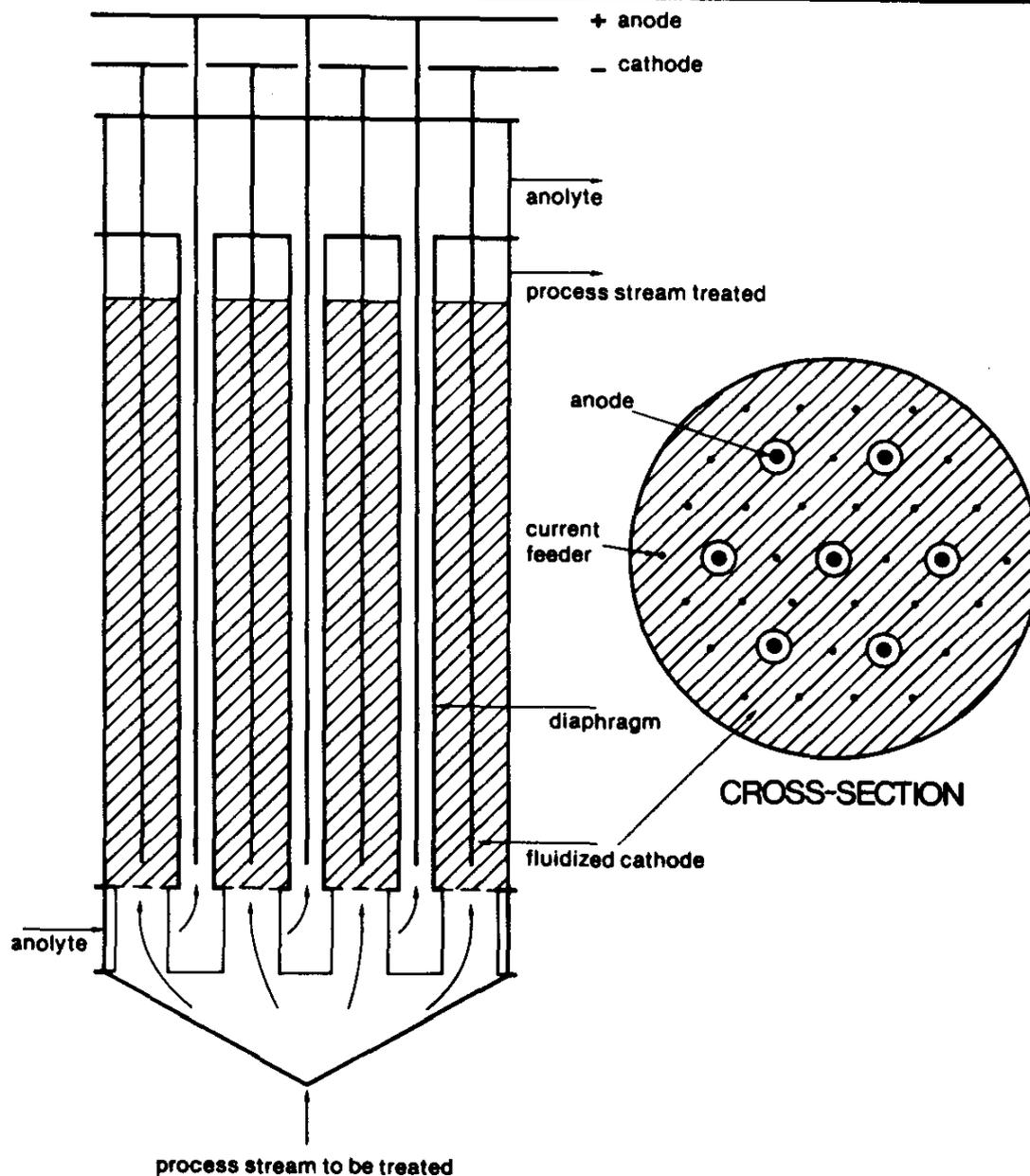
Figure 4. Cell Configuration of FBE Cell
