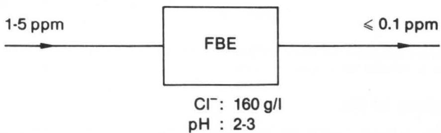
Figure 9. Mercury Removal from a Process Stream in a Mercury Cell Chlor-Alkali Electrolysis Plant
