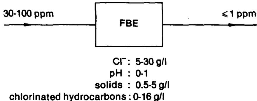
**Figure 7. Copper Removal from a Process Stream in a Plant for Chlorinated Hydrocarbons**
