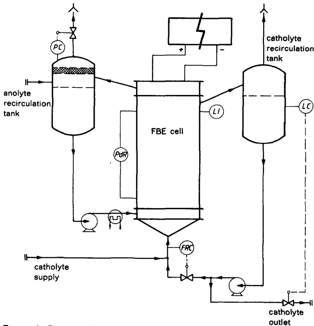
Figure 6: Process flow diagram of an FBE unit
